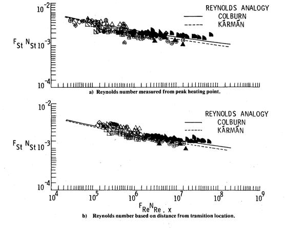
Fig. 1 Turbulent heat data transformed by the Eckert reference-enthalpy method and compared with the Schultz-Grunow relation.
